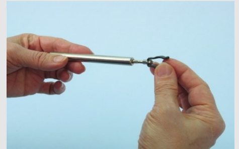
Insert force gauge holder into stand rod
