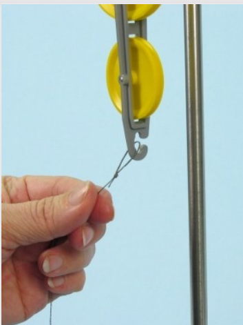
Fasten fishing line to the fixed reel
