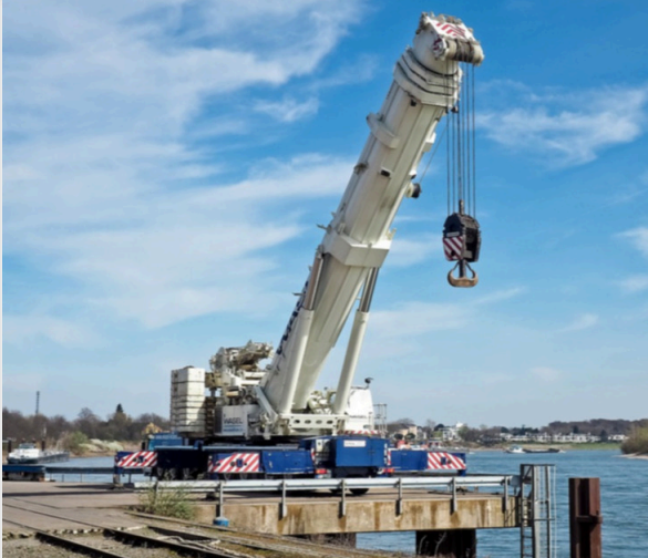
Crane with pulley block
